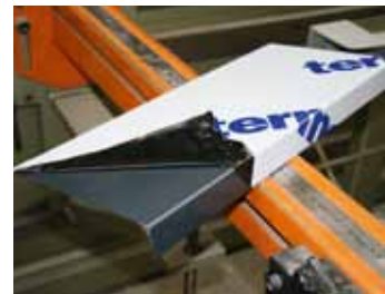
No cracking once coated
